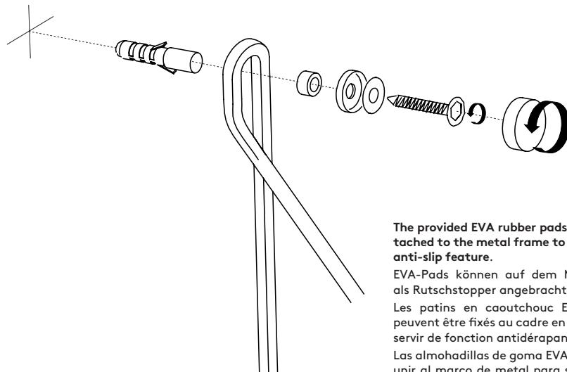
The provided EVA rubber pads can be attached to the metal frame to serve as an anti-slip feature.
