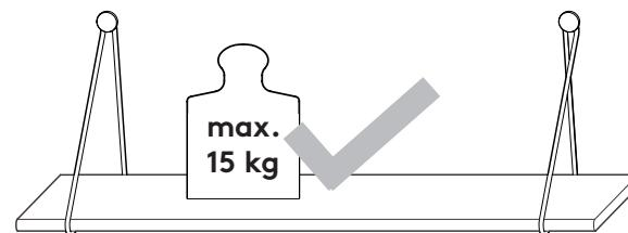
The supplied mounting hardware (screws/wall plugs) is suitable for walls out of brick, stone and concrete. For all other wall materials different hardware should be used.
